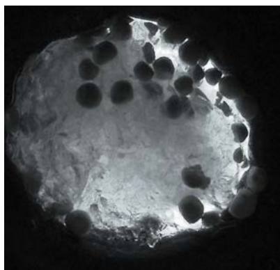
Figure 3- Photomicrograph of an SI-sphere (20x) post-conductivity test at 8000 psi closure stress
