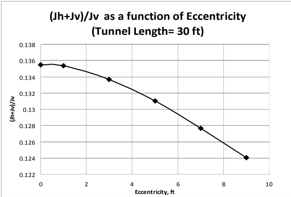
Figure 3 -  $(J_h + J_v) / J_v$  as a function of Eccentricity
