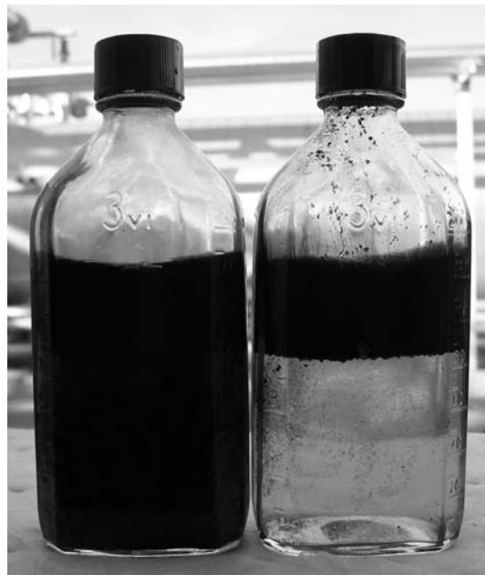
Figure 1 - The novel REB was specifically developed to treat production where a significant amount of the oil produced is carried by the produced water as a reverse emulsion. This particular type of emulsion occurs where high oil production is coupled with high water production, as in SAGD and other high-flow, primary-production fields around the world.
