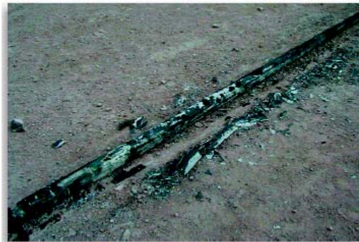
Figure 4 - Scale And Produced Solids Bonded to the ESP Motors Inside the Shroud Causing Excessive Heating And Motor "Burn Out"
