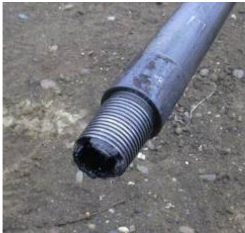
Picture 1 –PCPRod®1000 nipple turbulence wear
