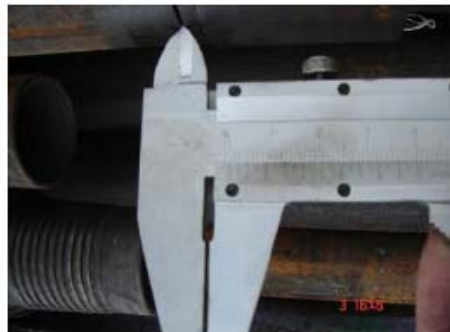
Picture 4 – Nipple connectors without over torque or galling and keeping the original stand off.
