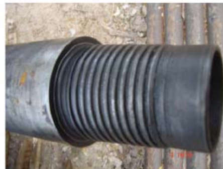
Picture 4 – Nipple connectors without over torque or galling and keeping the original stand off.
