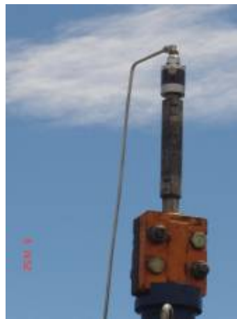
Picture 2 – Surface installation for injection through the HR while producing
