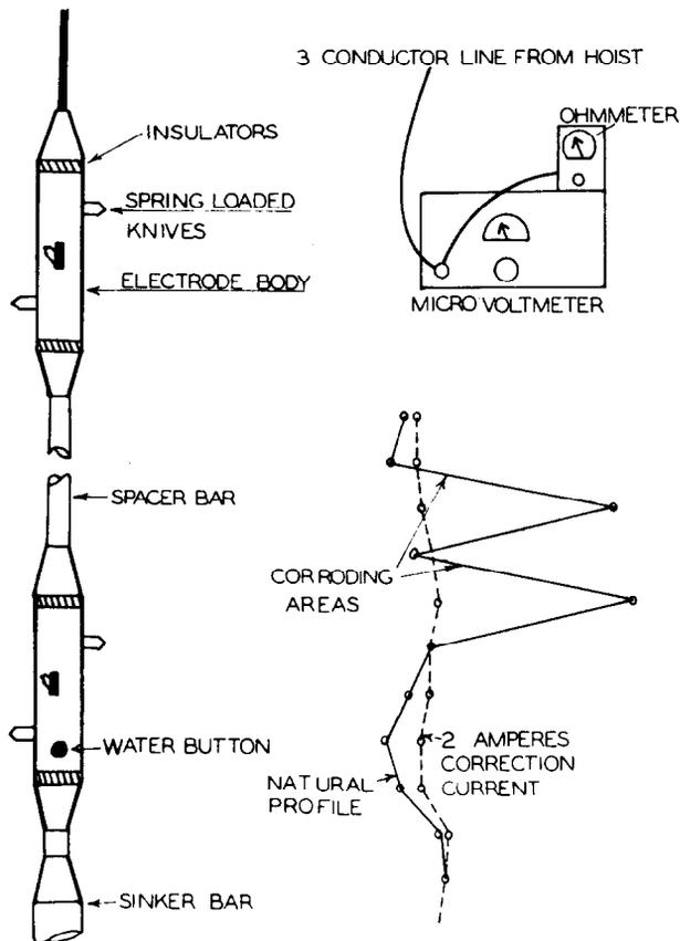
FIG 1 CASING POTENTIAL PROFILE (EQUIPMENT & RESULTS)
