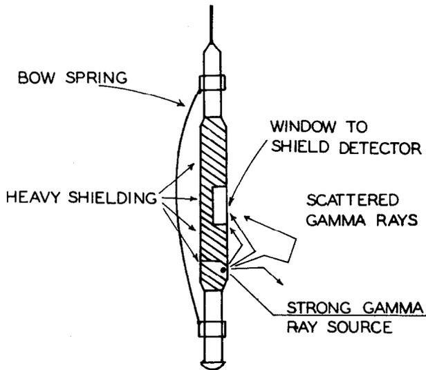
Fig. 2 DENSILOG INSTRUMENT
