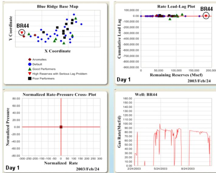
Figure 4 - The four performance plots in this figure are part of a multi-well management system for the Blue Ridge Field. The key plot in this instance is the Lead-Lag plot in the upper left. Note that Lead-Lag is plotted versus Remaining Reserves. This is part of an animation sequence. This particular plot is taken at the beginning of the sequence, or Day 1.
