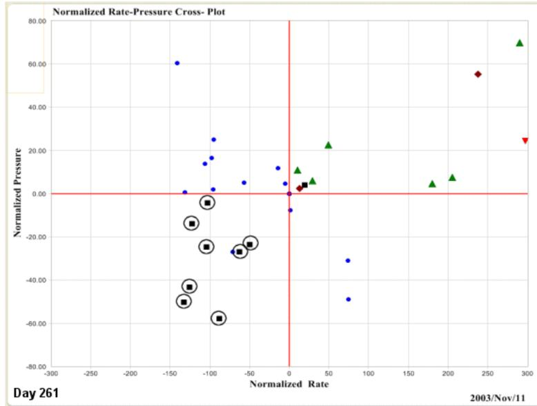
Figure 8 - This is the same Cross-Hair plot as shown in Fig. No. 5. The wells shown in the lower left quadrant all have unexpectedly low cumulative normalized rates and pressures and need further investigation. See Fig. No. 9 for further data of relevance to this problem.
