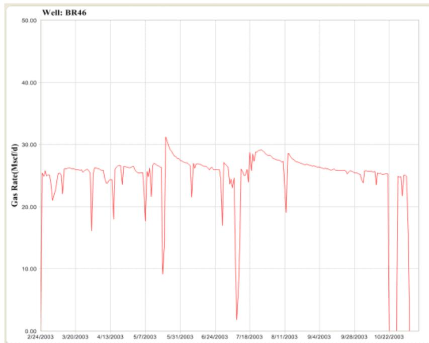
Figure 7 - This is the rate versus time plot taken from Fig. No. 5 for BR 46. The production rates for both this well and GB1 are not declining, even though the wells are indicated on the Lead-Lag plot to have very low reserves. This anomaly leads to the possible suspicion that these two wells have higher reserves than previously thought. Recommended Action: Re-evaluate the reserves in this area of the field.
