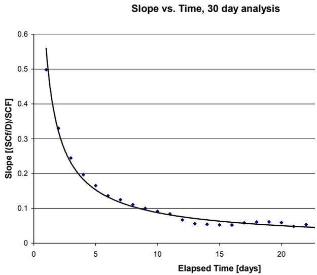
Figure 3 - This is the plot from which the best-fit slope function was generated. A number of time slices from Rate vs. Cum Production plots, such as that shown in Fig. No. 2, were used to generate Fig. No. 3. This slope function is for a short-term study with a 30-day time period. See the section titled Dynamic Baselines for more details.
