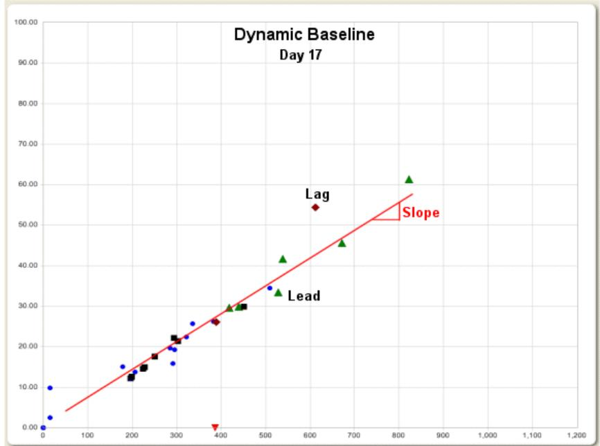
Figure 2 - This figure shows one time slice in the construction of a dynamic baseline. Rate is plotted on the Y-axis and cumulative rate on the X-axis. The red line represents the least squares, best-fit line. The slope of this line is used to generate a slope function as shown in Fig. No. 3. See the section titled Dynamic Baselines for more details.
