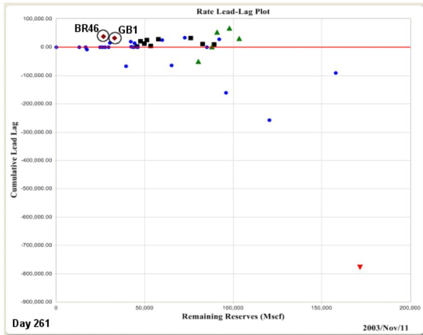
Figure 6 - This figure shows an expanded view of the Lead-Lag plot versus Remaining Reserves shown in Fig. No. 5. Using this plot and the others included in Fig. No. 5, the BR 46 and GB1 wells were discovered to have an interesting anomaly. Note that both wells are in a Leading position, but have some of the lowest remaining reserves. See Fig. No. 7 for a rate plot of BR 46 which identifies the anomaly.
