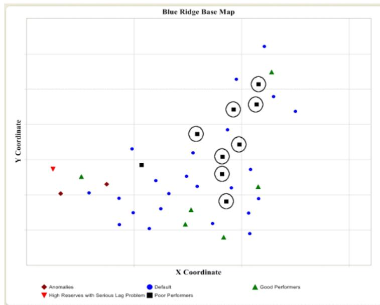
Figure 9 - This is the same Base Map as shown in Fig. No. 1. It shows the location of the poorly performing wells identified in Fig. No. 8. Note that they are all in the same area. Further investigation revealed that they were all connected to the same lateral and compression system.
