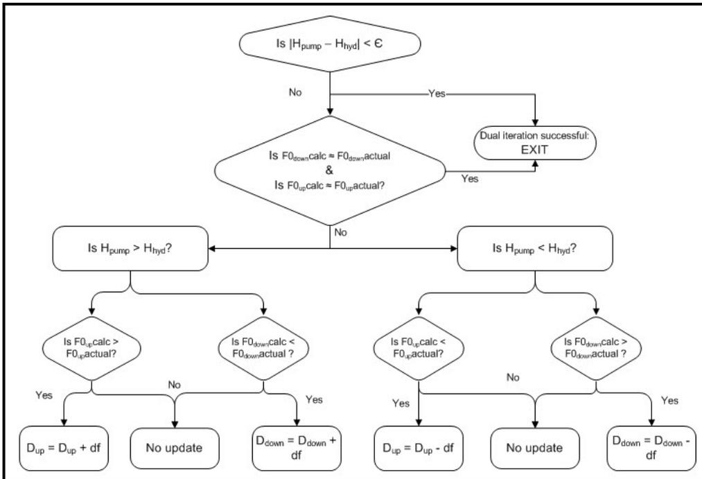
Figure 3 - Flowchart variation on the upstroke and downstroke damping criteria.
