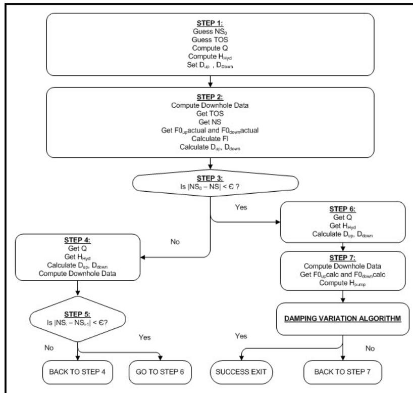
Figure 2 - Flowchart for the dual iteration on the net stroke and damping factors for the modified Everitt-Jennings algorithm.
