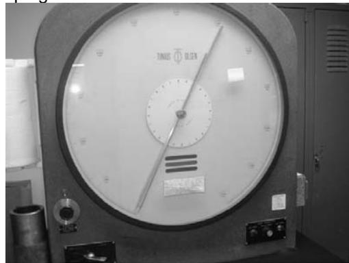
Figures C & D - Compressive Strength Tester [0 – 12,000 psi] – Utilized to Perform Flat Plate Extrusion Testing
