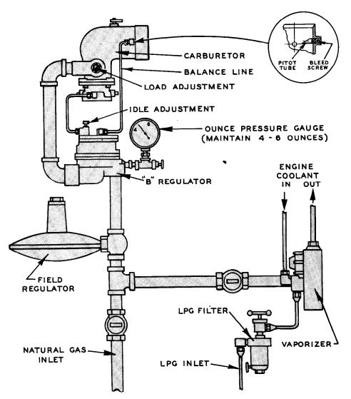
The purpose of the field regulator is to reduce the gas supply line pressure to a valve low enough to be easily controlled by the sensitive "B" regulator. Four to six ounces pressure is required at the inlet to the "B" regulator, regardless of engine size, speed, or load.
