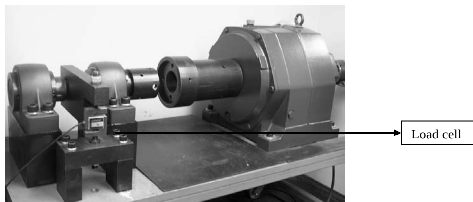
Figure 3 - Displacement Testing Machine with the Load Cell
