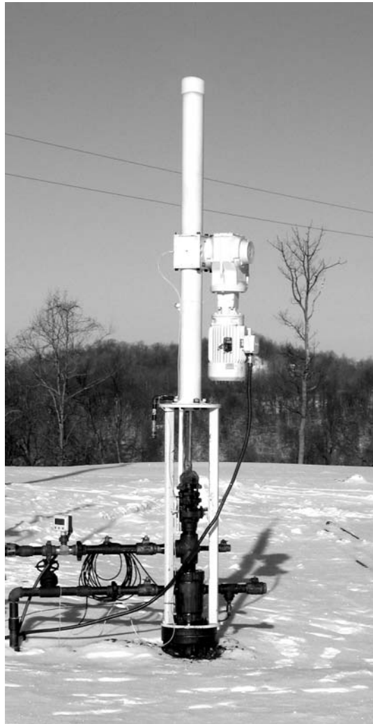
Figure 1— LRP® Linear Rod Pump
