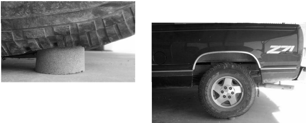
Figure 3—A simple test of LRS-coated sand pack after curing and obtaining sufficient consolidation strength to withstand stress loading.
