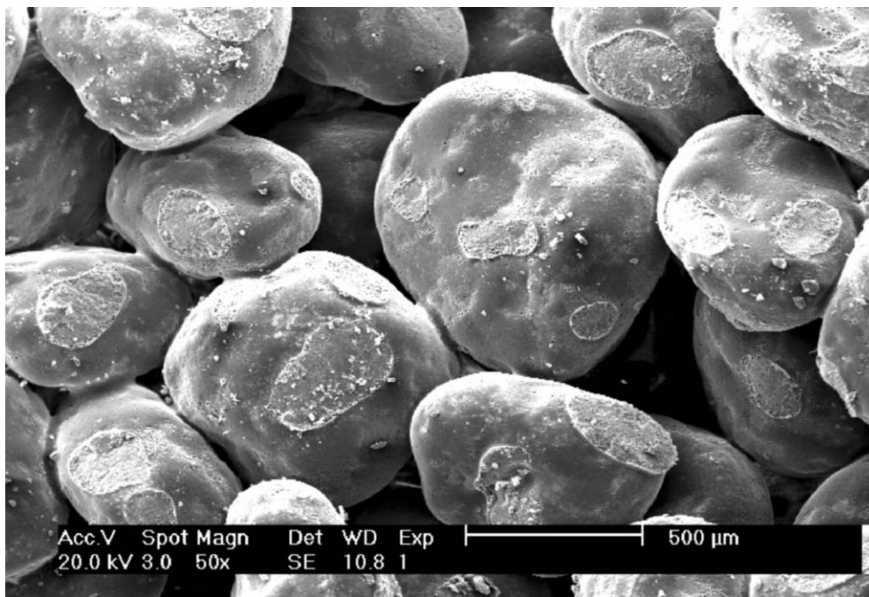
Figure 2—Photomicrograph (50X) of 20/40-mesh Brady sand that has been coated with LRS.
