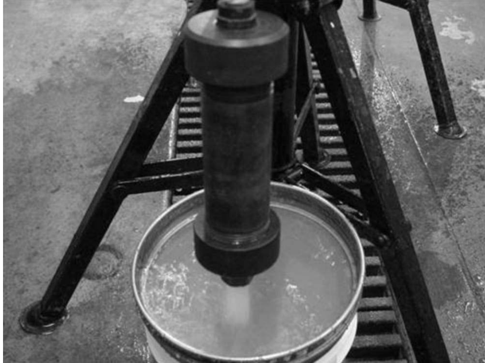
Figure 5—A flow cell was used in packing LRS-treated 20/40-Brady sand, curing at temperature, and pumping water through the pack at various flow rates to determine the resin performance in controlling flowback of the consolidated sand pack.
