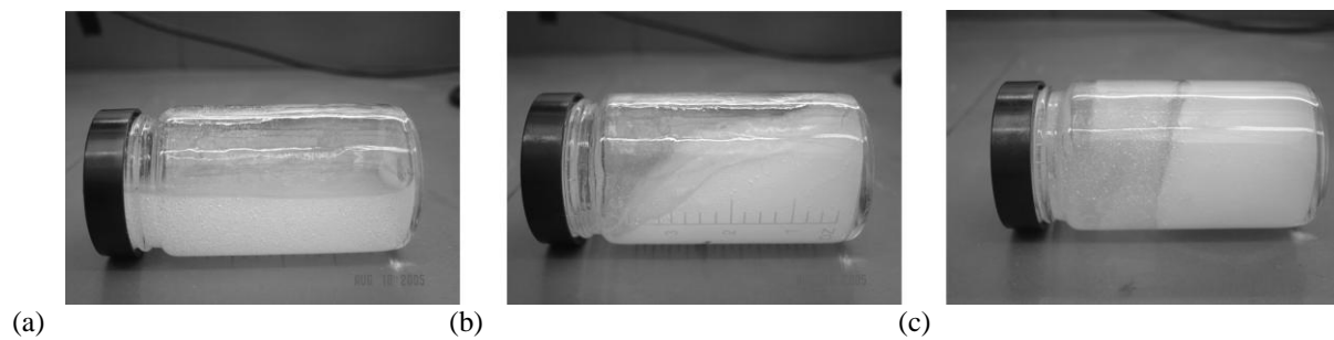
Figure 2 - Physical appearance of TIPG: (a) system has not developed thixotropic properties yet; (b) system has started developing thixotropic properties but it still slumps; and (c) ideal state of TIPG system (no slumping when movement stops).
