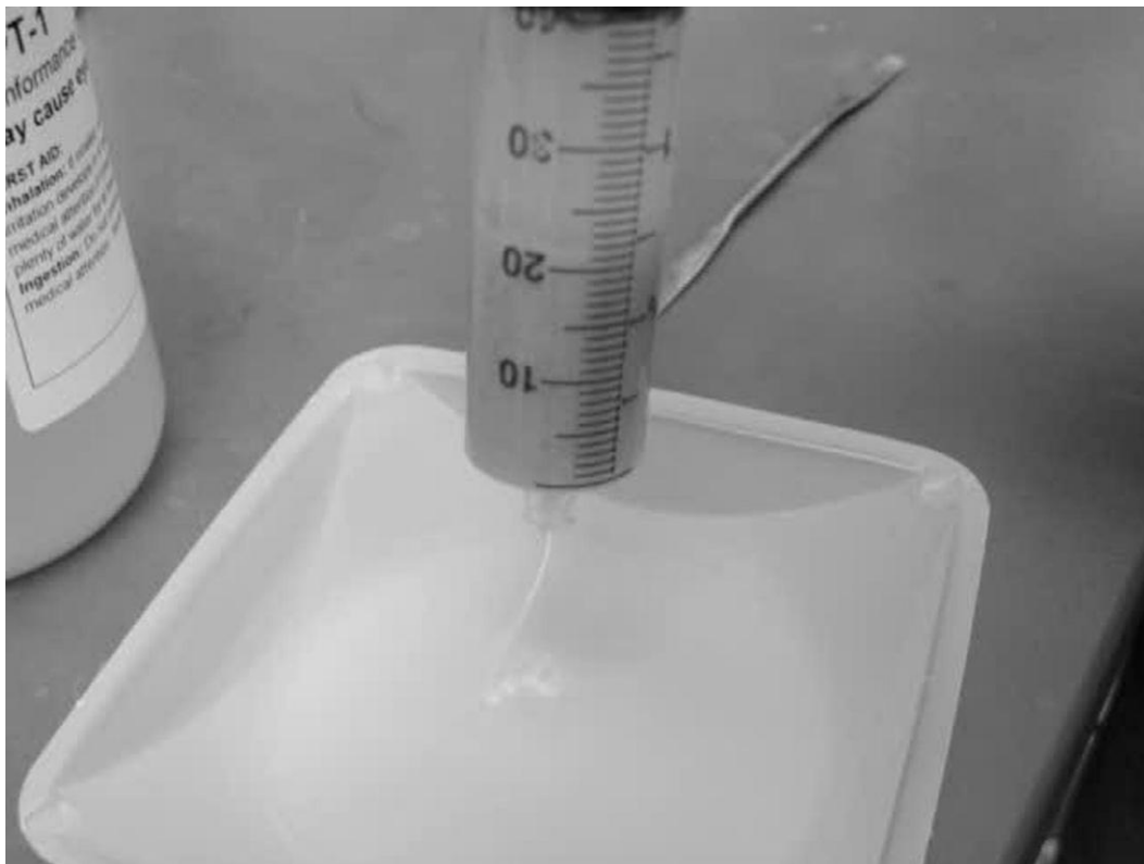
Figure 14 - TIPG System Being Filtered Through a 1.5-in. 20/40 Sand and 125-Micron Screen at 180°F
