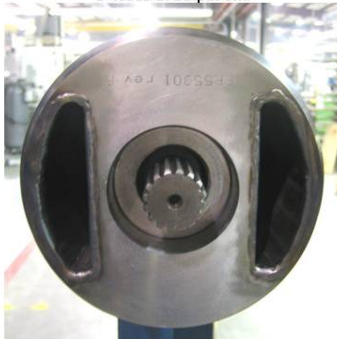
Figure 5 Photo of GCP Transmission D-tubes at output end
