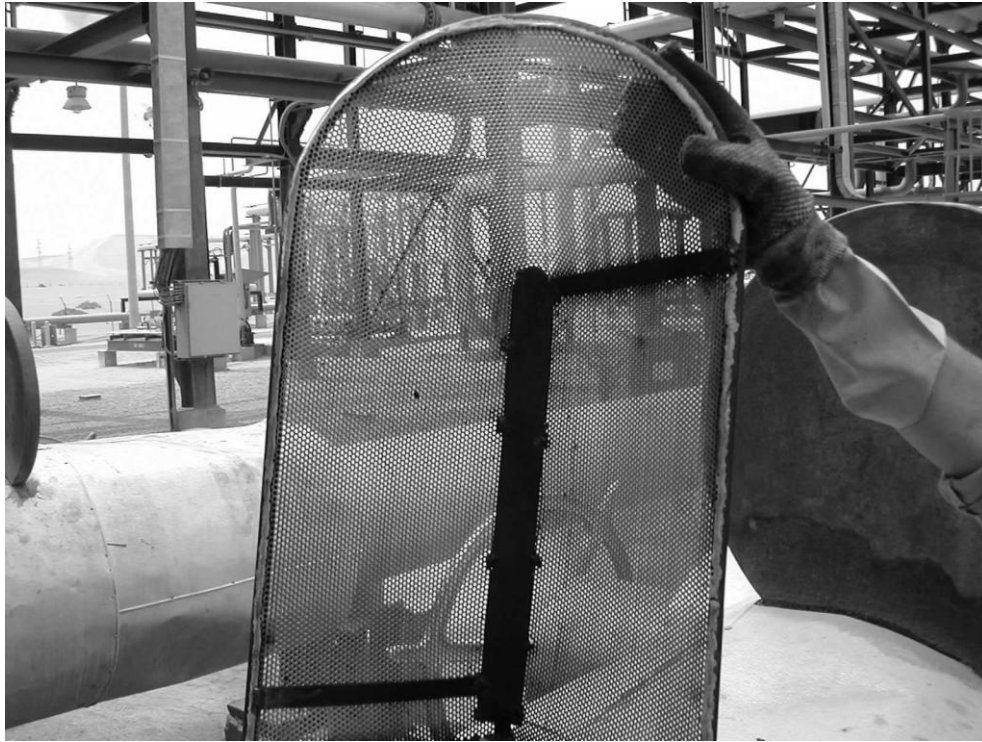
Figure 3 - Train 1 Stabilizer Pump Strainer After 30 – 40 ppm Inhibitor C Scale Inhibitor Treatment
