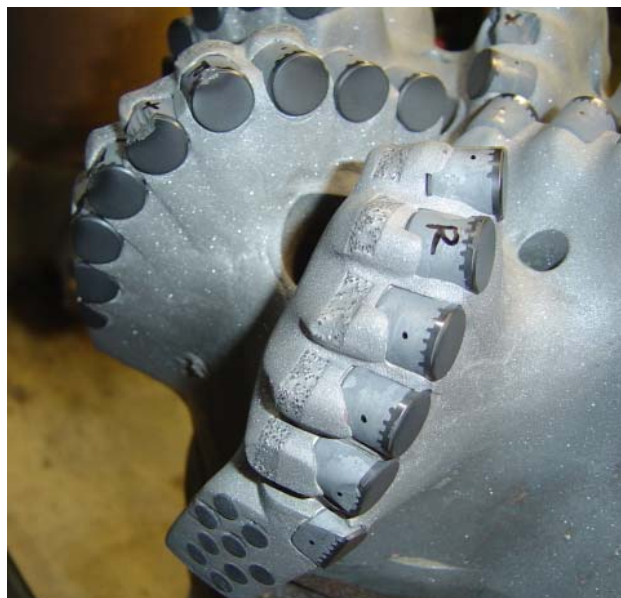
Figure 9 – Dull FM2745R after Drilling Entire 7 7/8-in. Interval of 8,860 feet in 126.5 hours at an average of 70 ft/hr.
