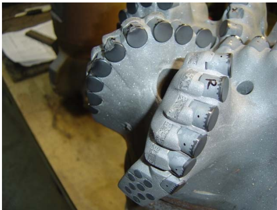
Figure 4 and Figure 5 – Impact Arrestors to Dampen Axial Vibration Impreg disks within arrestors are visible in Figure 4.
