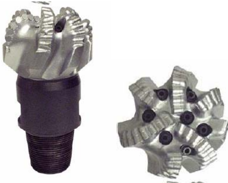
Figure 3 – Initial PDC Bit Design – FM2745
