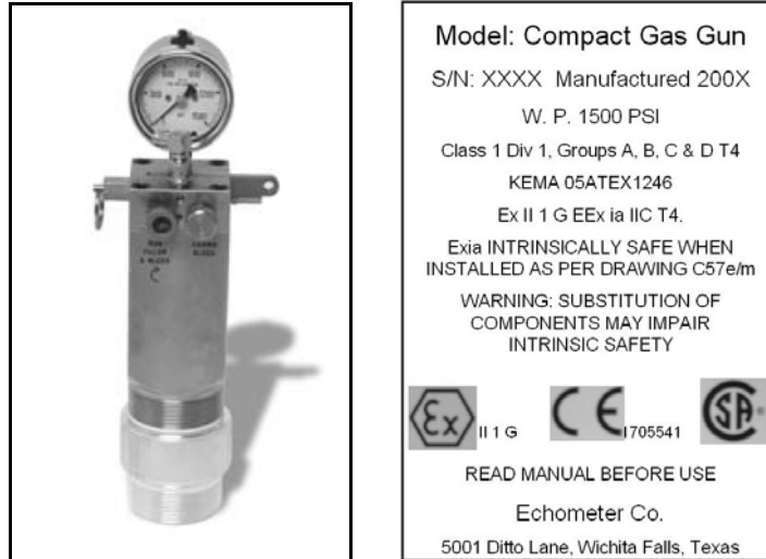
Figure 1 - Compact Gas Gun Modified (as shown by the engraving) with Special Microphone for Use in Hazardous Areas
