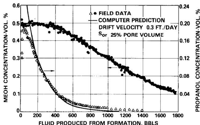
FIG. 2 METHANOL AND ISOPROPANOL CONCENTRATION PROFILES FROM TEST A.
