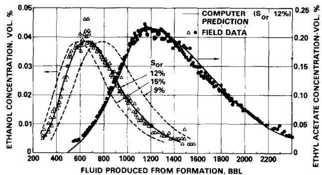
FIG. 6—ETHANOL AND ETHYL ACETATE PROFILES FROM TEST B.
