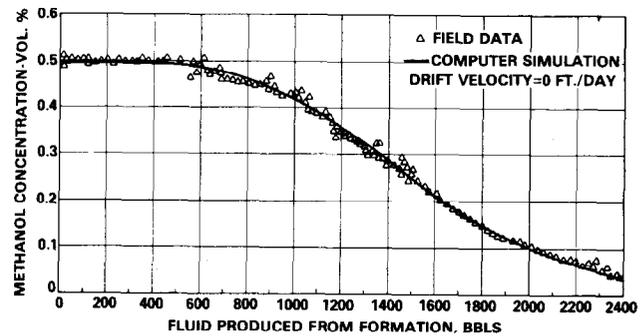
FIG. 5 — METHANOL CONCENTRATION PROFILE FROM TEST B.
