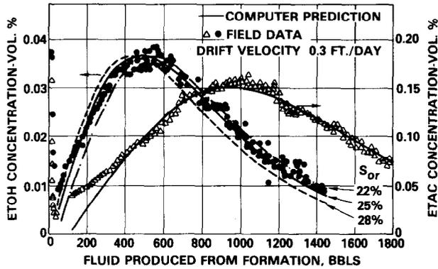
FIG. 3—ETHANOL AND ETHYL ACETATE CONCENTRATION PROFILES FROM TEST A.
