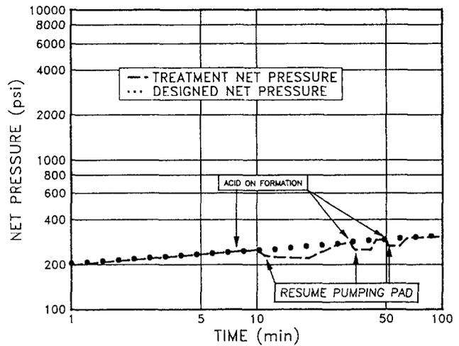
Figure 4 — Typical net pressure response with alternating pad and acid stages
