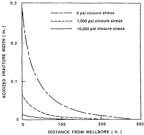
Figure 1 — Acidizing fracture width as a function of the distance from the wellbore and closure stress (from Novotny, 1977)
