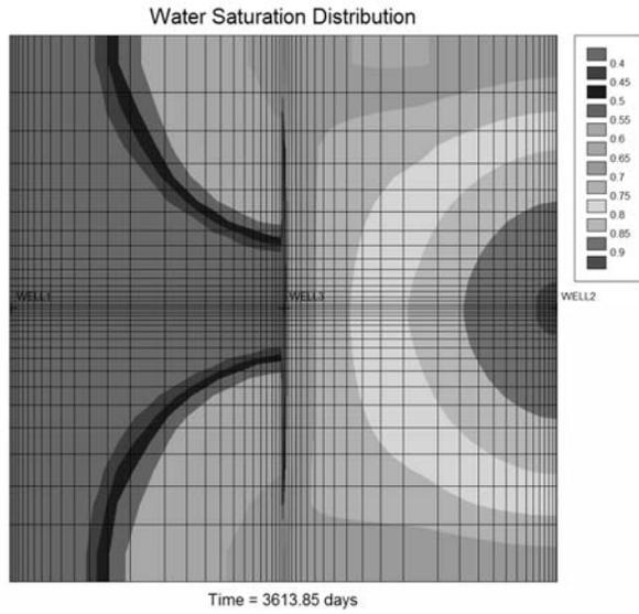
Figure 12—Planar Water Saturation Distribution in the Presence of a Barrier Fracture
