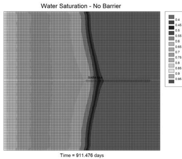
Figure 8—Water Breakthrough into the Horizontal Well When No Barrier Exists
