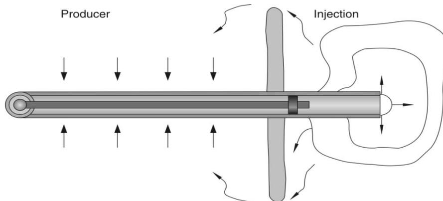
Figure 1—Injection and Production using a Single Wellbore, After Sierra et al. 2010
