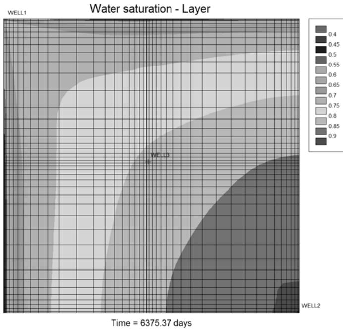
Figure 18—Water Saturation Distribution in the Absence of a Barrier Fracture
