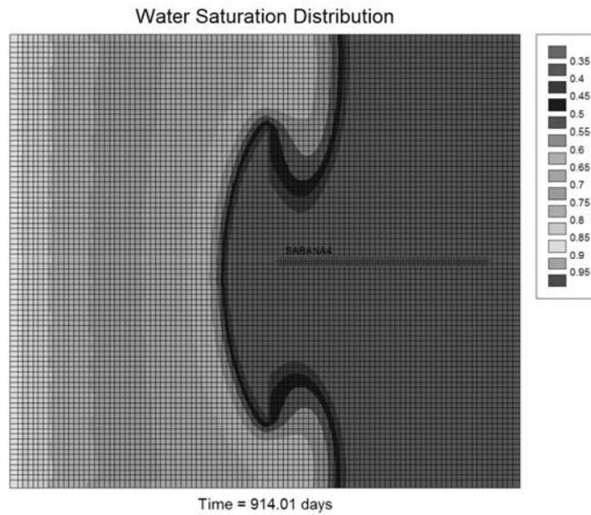
Figure 9—Water Breakthrough into the Horizontal Well in the Presence of a Barrier Fracture
