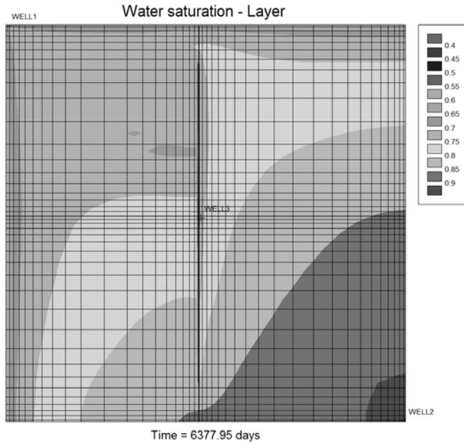
Figure 17—Water Saturation Distribution in the Presence of a Barrier Fracture
