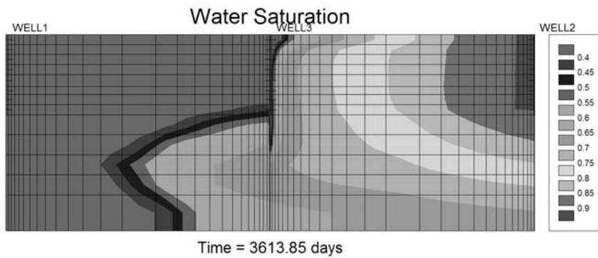
Figure 13—Cross-Sectional Water Saturation Distribution in the Presence of a Barrier Fracture
