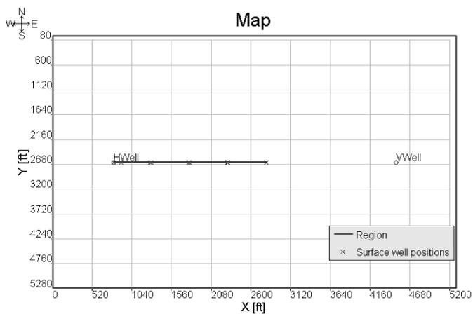
Figure 2—Map of Horizontal Producer with Vertical Injector, After Sierra et al. 2010
