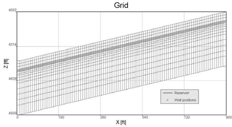
Figure 7—Reservoir Grid with Edge Water Drive
