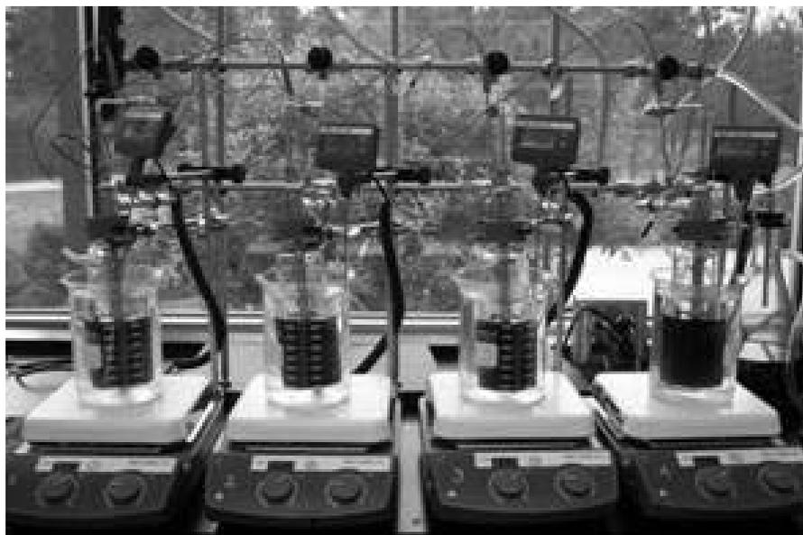
Figure 8 - Photograph of the four cell cold finger apparatus used during testing. The chiller bath is out of view on the right-hand side.
