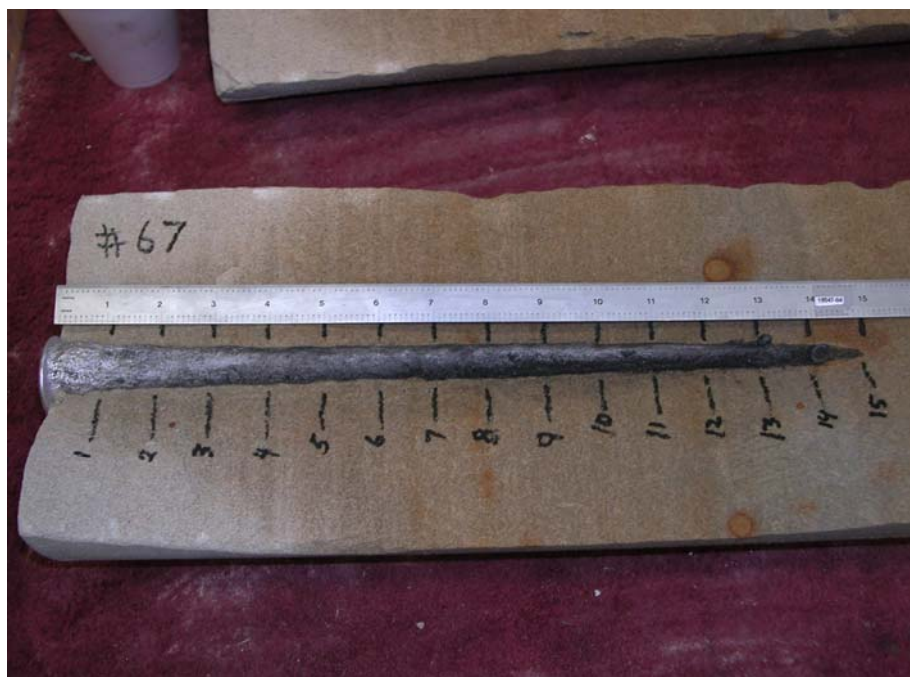
Figure 7b - Core Shot at 3500 psig Underbalance.
