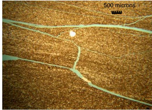
Figure 10 - Morrow Shale Exposed to West Texas Brine After 6 Hours
