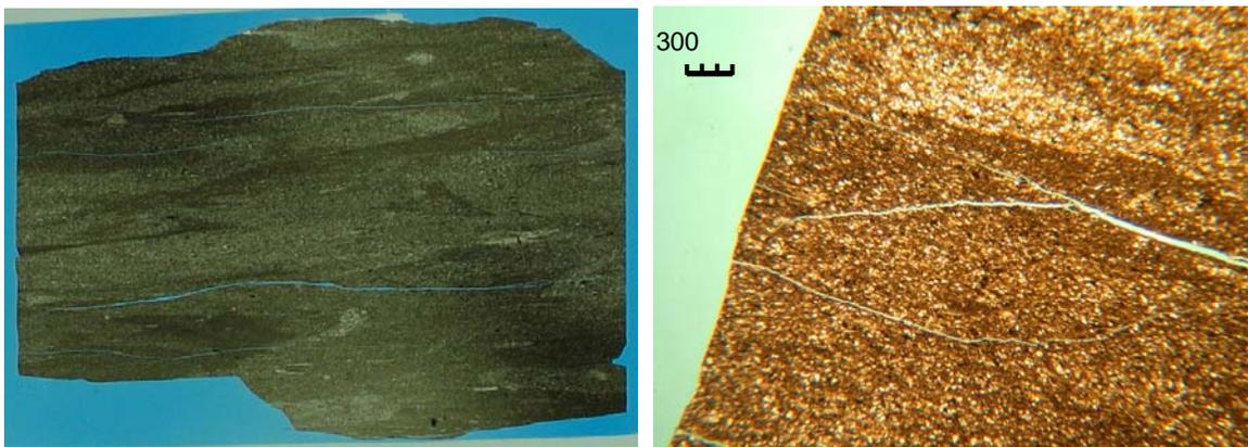
Figure 9 - Morrow Shale Exposed to 12 PPG K-Formate Brine After 6 Hours
