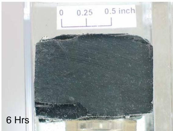
Figure 4 - Morrow Shale Exposed to 12 PPG K-Formate Brine
