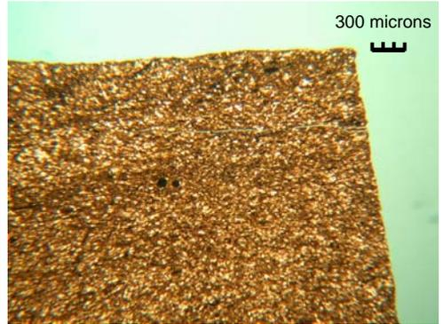
Figure 11 - Morrow Shale Exposed to Diesel After 6 Hours
