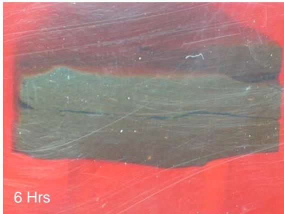
Figure 6 - Morrow Shale Exposed to Diesel
