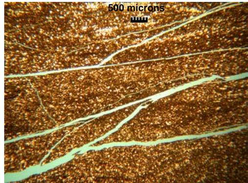
Figure 12 - Morrow Shale Exposed to Water After 6 Hours
