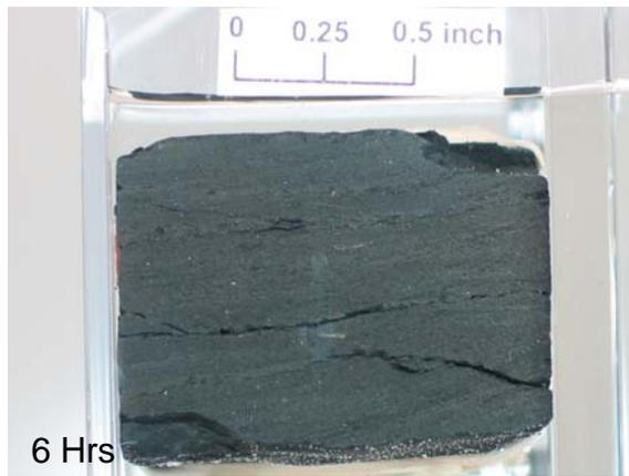
Figure 5 - Morrow Shale Exposed to West Texas Brine
