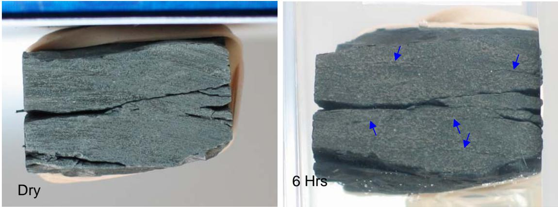
Figure 7 - Morrow shale exposed to water. Arrow indicate fractures.
