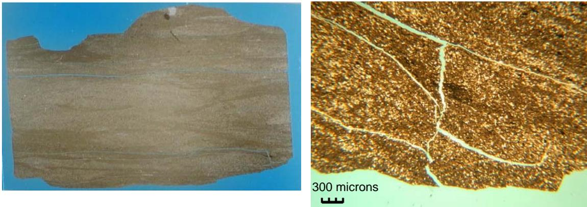
Figure 8 - Morrow shale exposed to 6% KCl Brine after 6 hours. The picture on the left side represents the whole thin section of the tested sample and on the right side represents part of the thin section which was observed through microscopy in this figure and the following.
