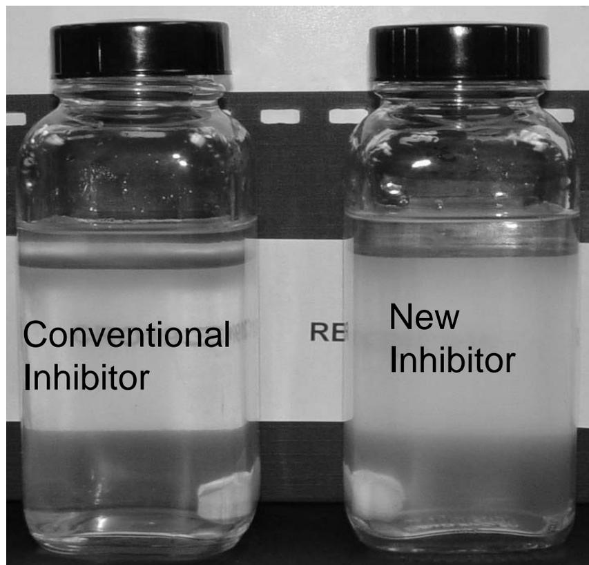
Figure 4 - Dispersibility of corrosion inhibitors after 1 hr of mixing. (2,000 ppm inhibitor in CO<sub>2</sub> saturated solution, Isopar M/NACE brine, 10/90).
