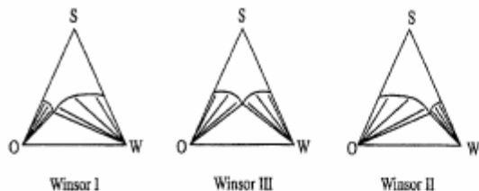
Figure 1. Schematic of ternary phase diagrams for Winsor microemulsions. In the left-hand shaded area, the microemulsion is in equilibrium with excess water, and in the right-hand shaded area, the microemulsion is in equilibrium with excess oil. The Winsor III microemulsion is in “middle phase” with an excess of both water and oil [2].
