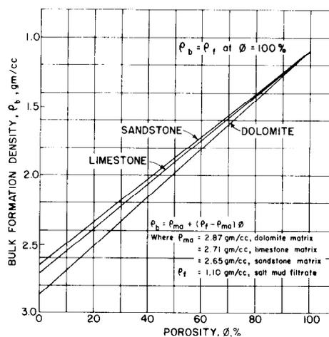
FIGURE 4—BULK FORMATION DENSITY VS. POROSITY COMPARING VARIOUS MATRIX DENSITIES
