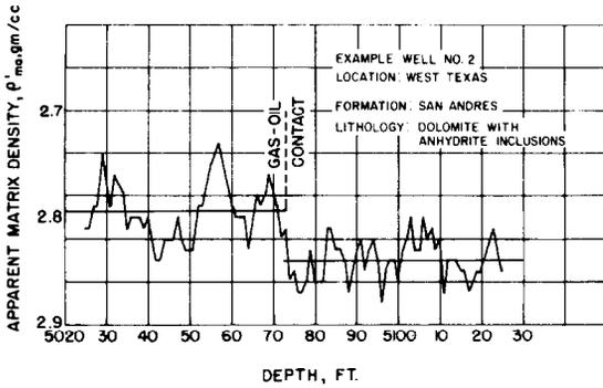
FIGURE 8—APPARENT MATRIX-DENSITY CROSS-PLOT
