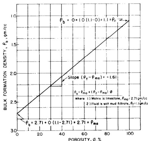
FIGURE 3—BULK FORMATION DENSITY VS. POROSITY
