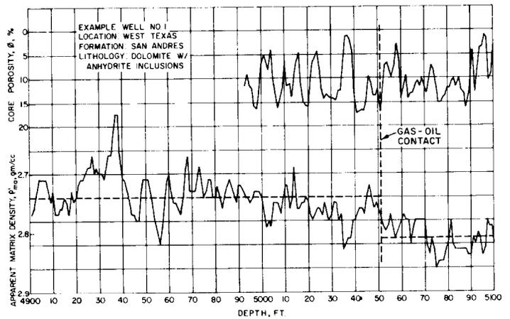
FIGURE 10—EXAMPLE WELL NO. 1, APPARENT MATRIX DENSITY VS. DEPTH
