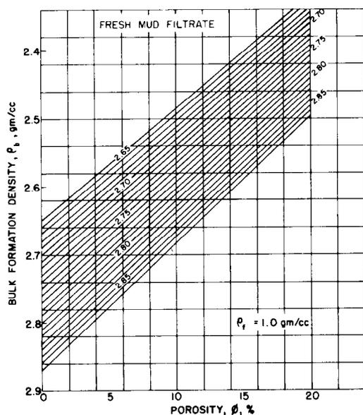
FIGURE 6—MATRIX-DENSITY CROSS-PLOT FOR A FAMILY OF MATRIX DENSITIES ( $\rho_f = 1.0$  gm/cc).
