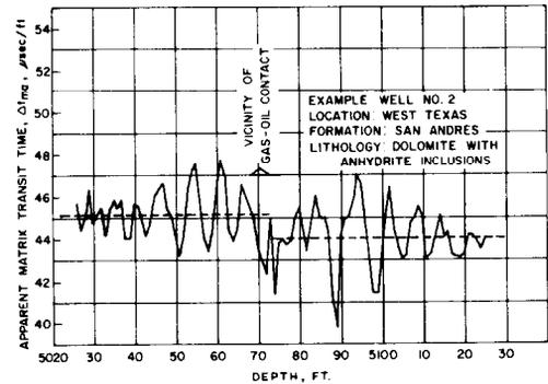
FIGURE 14—APPARENT MATRIX TRANSIT TIME VS. DEPTH
