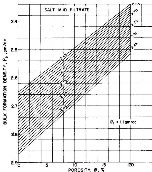
FIGURE 5—MATRIX DENSITY CROSS-PLOT FOR A FAMILY OF MATRIX DENSITIES ( $\rho_f = 1.1$  gm/cc).
