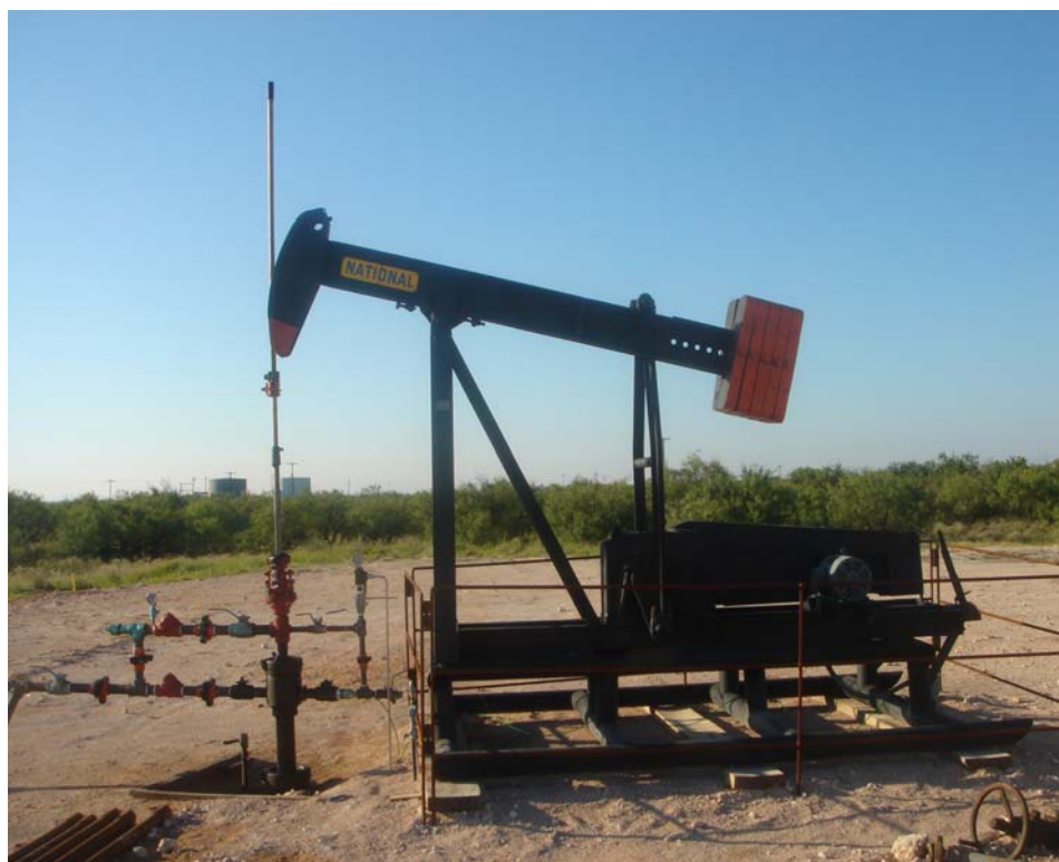
Figure 1 - National C25-65-24" Pumping Unit
