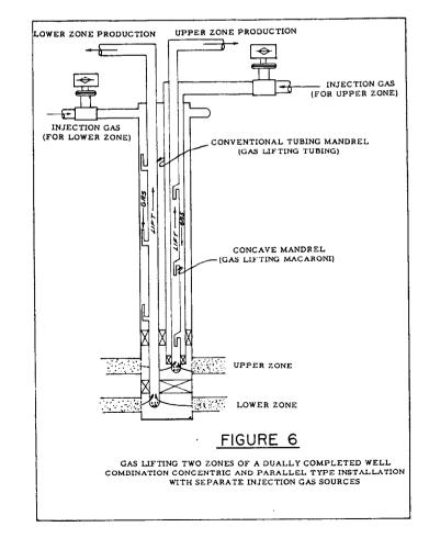
mandrels are designed to be run in 5-1/2" O. D. —17 lb. casing.
