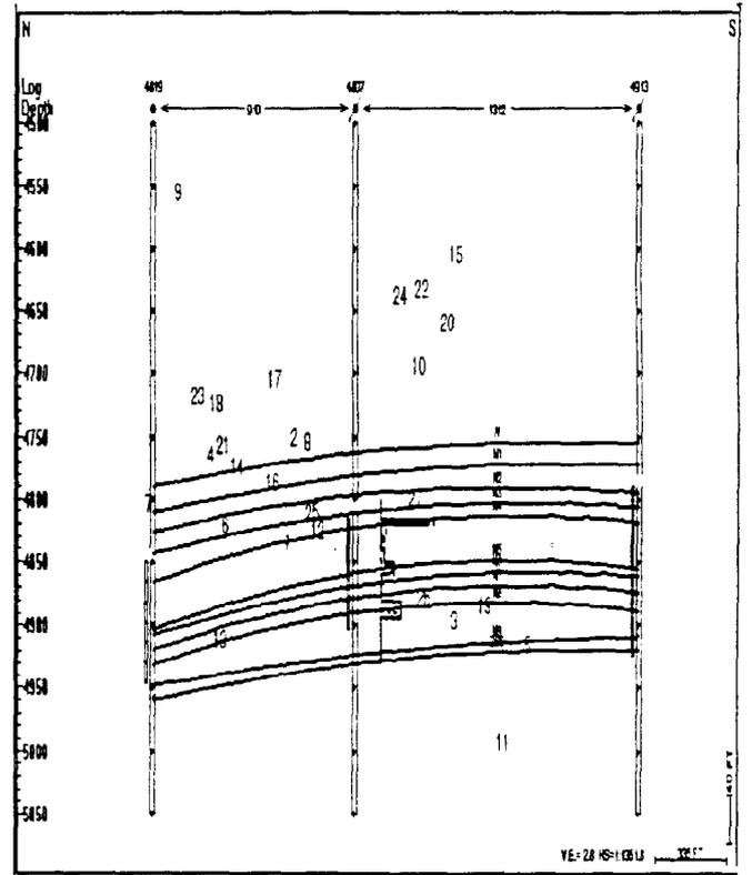
Figure 7 - Cross section of seismic events numbered as they occurred.
