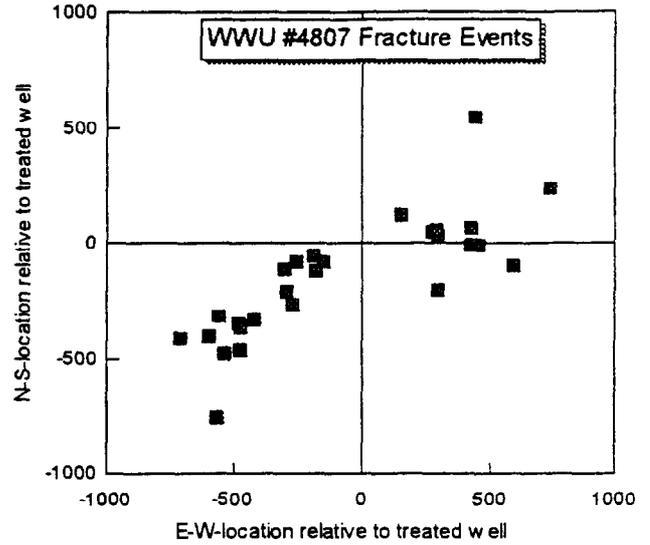
Figure 5 - Plan view of the seismic event locations.
