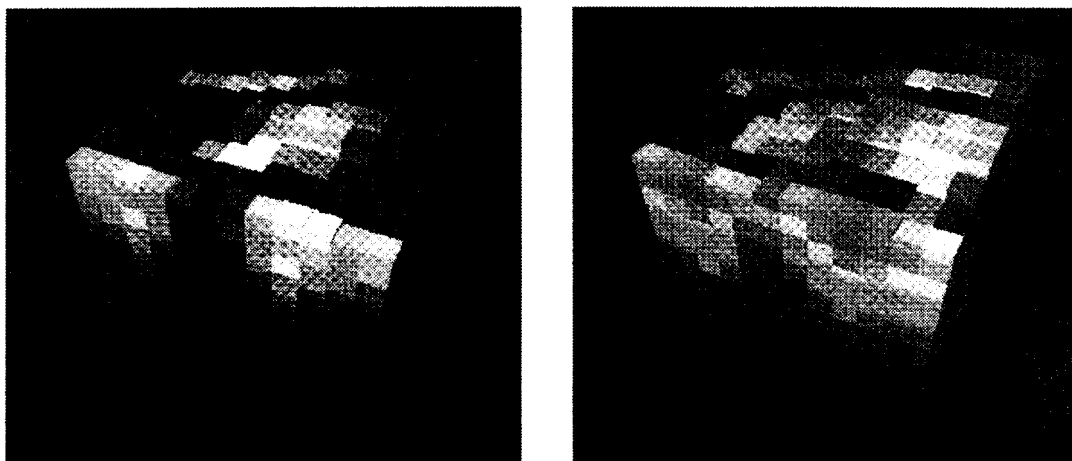
Figure 9 - Thermal Reservoir Model Temperatures at 1 Year and 3 Years of Steam Injection Model is cut along a fracture trend, where lighter shading reveals heating up to 470°F (darker cells remain at original temperature -82°F). Elevated temperature reveals areal and vertical heat movement along fracture trends.
