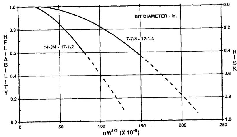
Figure 8 - Bearing reliability and risk of failures for two families of bits with metal-face seals
