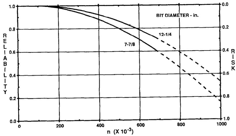
Figure 6 - Bearing reliability and risk of failure vs. bit revolutions for 7-7/8 and 12-1/4 in. bits with metal-face seals
