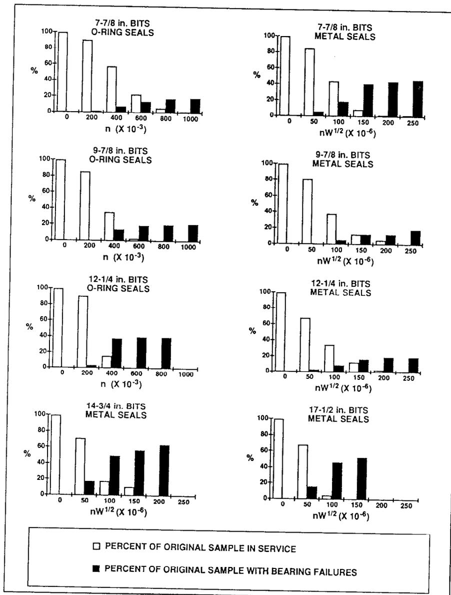
Figure 4 - Distributions of use and bearing failures for bit samples listed in Table 1
