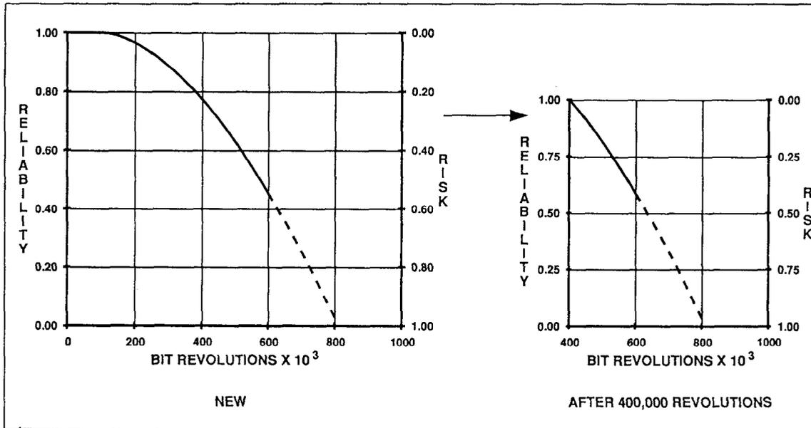
Figure 9 - Reliability of new and used 9-7/8 in. bits with O-ring seals
