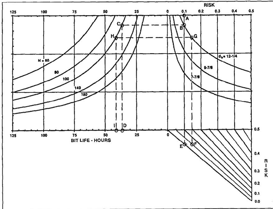
Figure 12 - Bearing life and risk forecast chart for bits with O-ring seals
