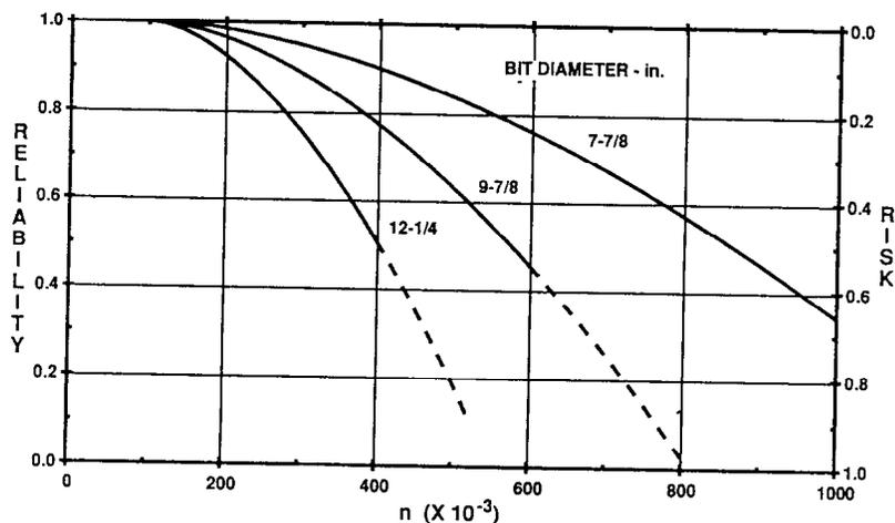
Figure 5 - Bearing reliability and risk of failure for bits with O-ring seals
