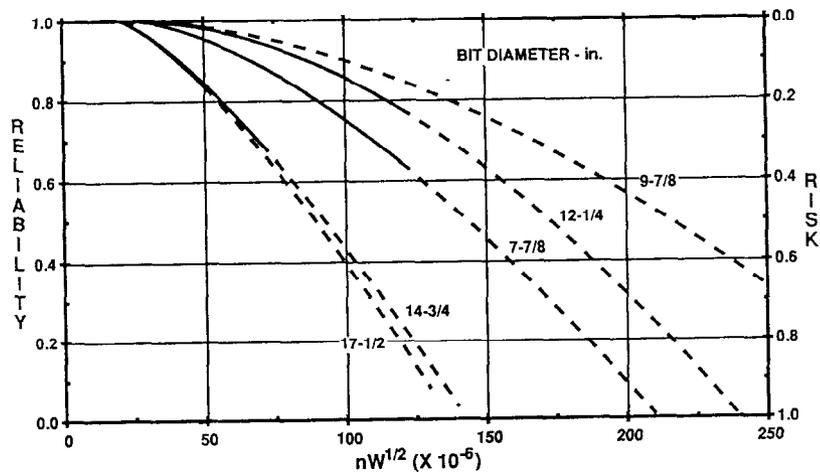
Figure 7 - Bearing reliability and risk of failure for bits with metal-face seals
