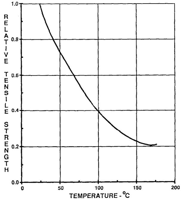
Figure 3 - Tensile strength vs. temperature for a typical rock bit O-ring seal
