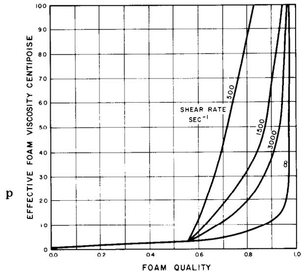
FIG. 4—EFFECTIVE VISCOSITY OF FOAM
