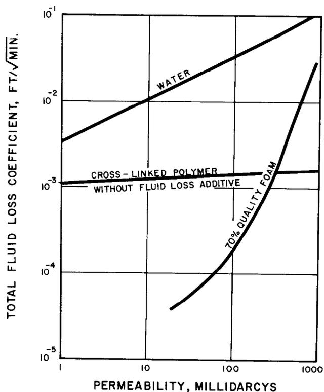
FIG. 5—TOTAL FLUID LOSS COEFFICIENT FOR FOAM, WATER, AND CROSS-LINKED POLYMER
