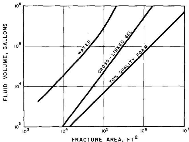
FIG. 7—FRACTURE AREA CREATED WITH VARIOUS FLUIDS
