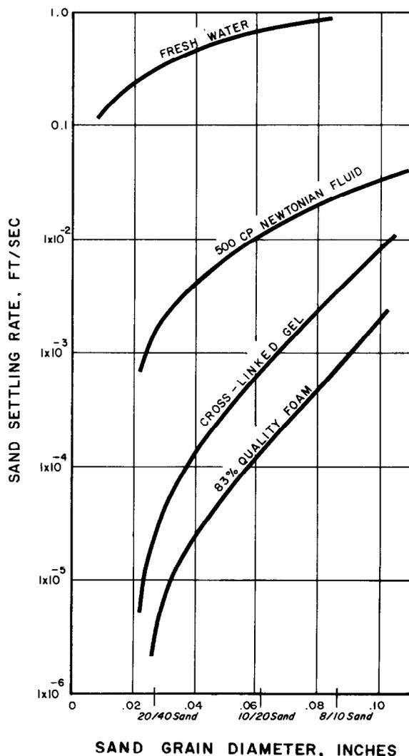
FIG. 6—SAND SETTLING VELOCITY OF SAND IN STATIC FOAM AND OTHER FLUIDS
