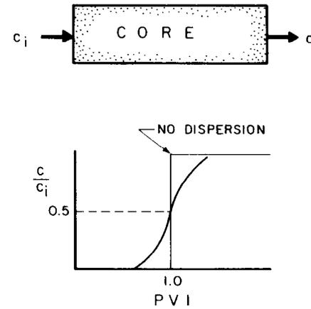
Figure 8 - Definition of tracer dispersion
