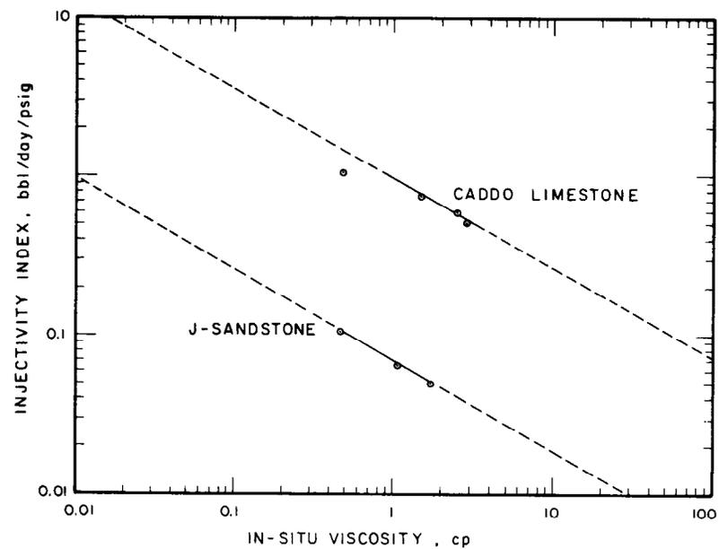
Figure 13 - Injectivity index, in-situ viscosity correlation
