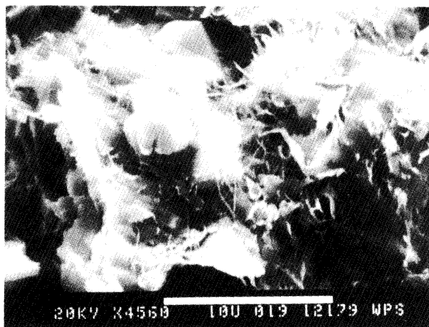
FIGURE 8—A HIGH MAGNIFICATION VIEW OF A LAYER OF ILLITE/MONTMORILLONITE OVERGROWTH ON QUARTZ SHOWING DELICATE, NEEDLE LIKE CLAY PROJECTIONS.
