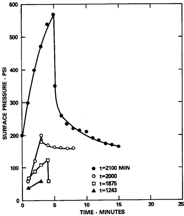
Figure 5 - Surface pressure on annulus during and after times that fluid was pumped in - Well B
