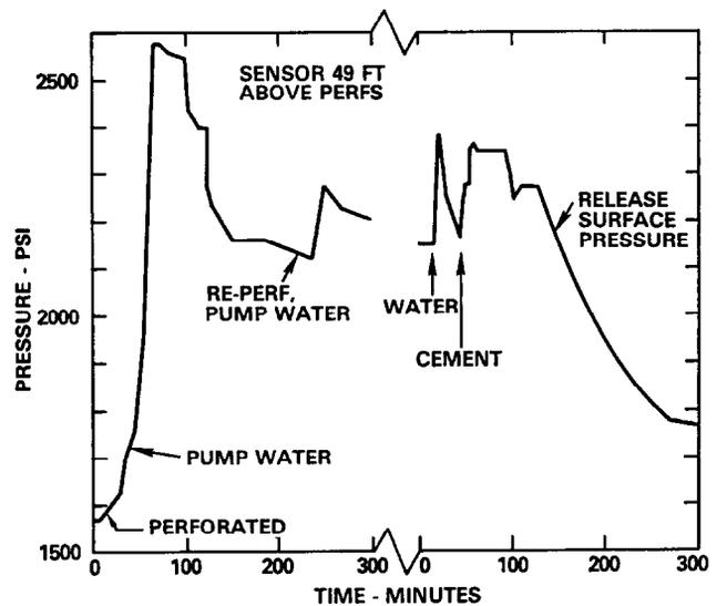
Figure 8 - Pressure response during remedial cementing - Well E
