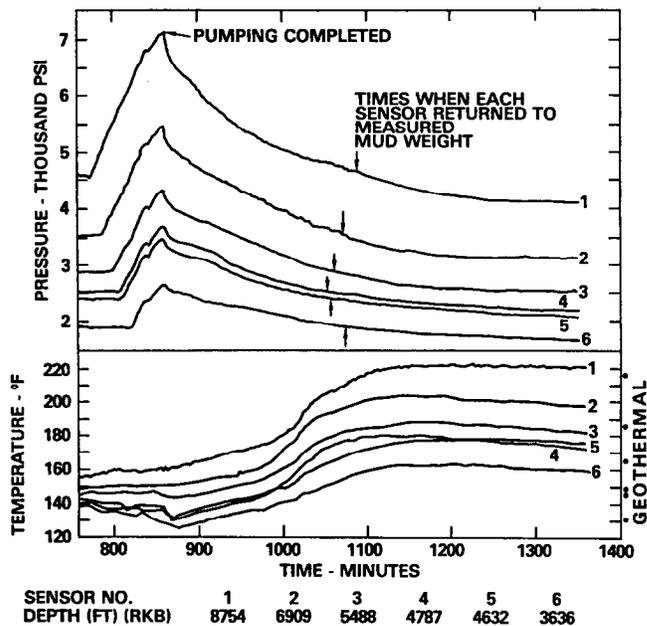
Figure 2 - Annular pressure and temperature - Well A
