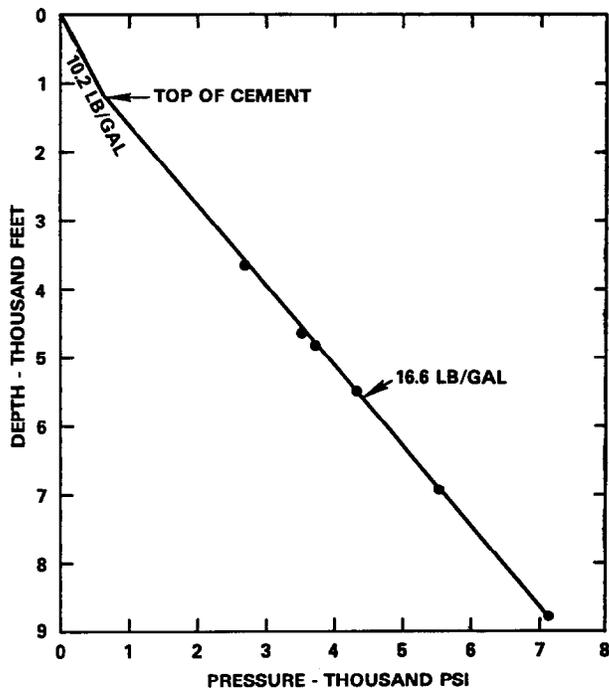
Figure 3 - Pressure vs. depth when cement pumping ended - Well A
