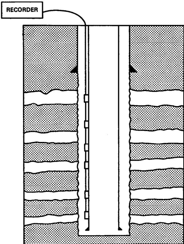
Figure 1 - Wellbore with sensors on casing
