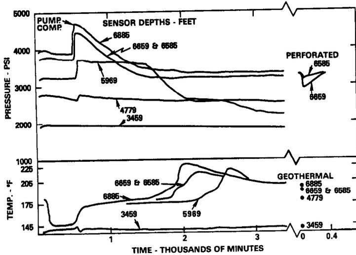
Figure 7 - Annular pressure and temperature - Well D
