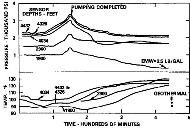
Figure 9 - Annular pressure and temperature
