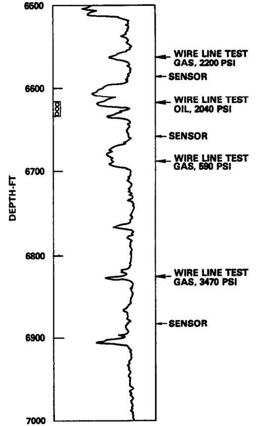
Figure 6 - Log, pore pressures, perforations, and sensor locations - Well D
