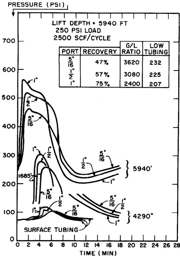
FIG. 15. COMPARATIVE PRESSURE RECORDINGS OF 5/16", 1/2" AND 1" PORTS (250 PSI LOAD).
