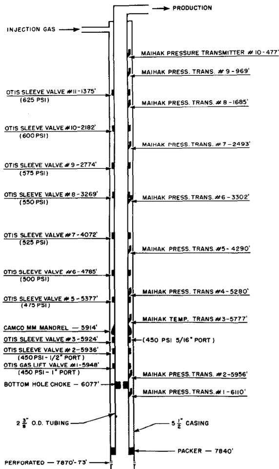
FIG. 2. DOWN-HOLE EQUIPMENT.
