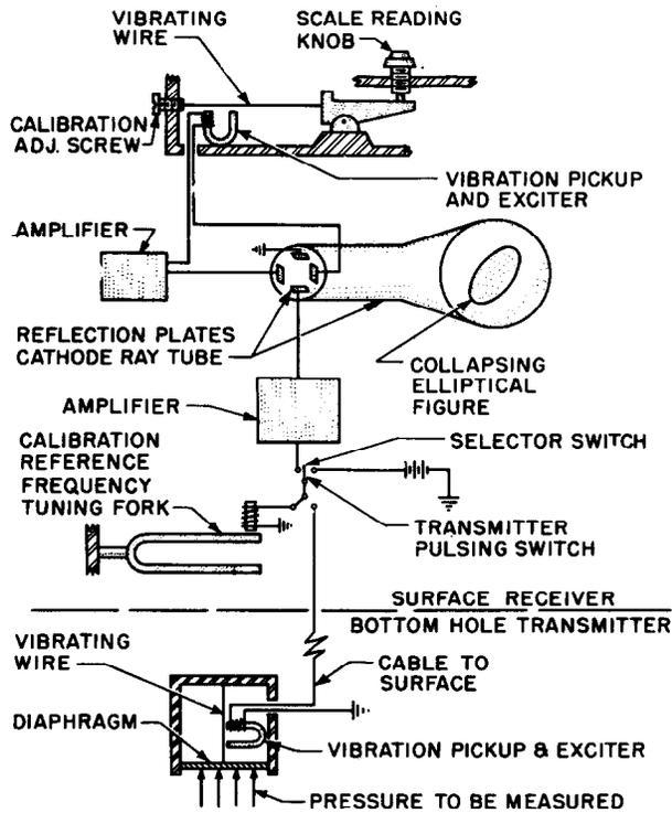
FIG. 5. SCHEMATIC DIAGRAM OF MAIHAK INSTRUMENTS.
