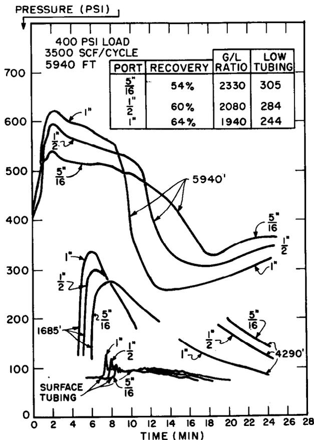
FIG. 18. COMPARATIVE PRESSURE RECORDINGS OF 5/16", 1/2" AND 1" PORTS (400 PSI LOAD).
