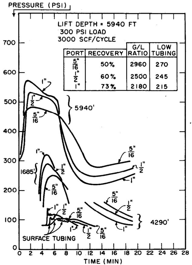
FIG. 16. COMPARATIVE PRESSURE RECORDINGS OF 5/16", 1/2" AND 1" PORTS (300 PSI LOAD).
