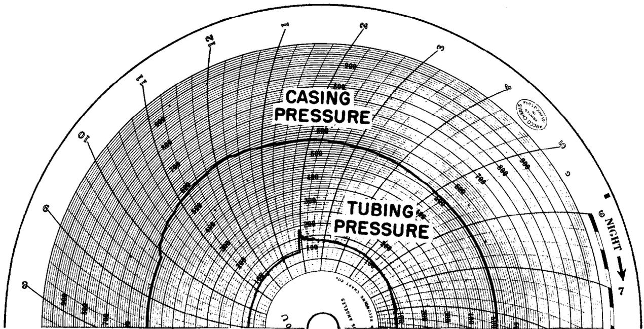
FIG. 6. 24 MIN. REVOLUTION RECORDING CHART
