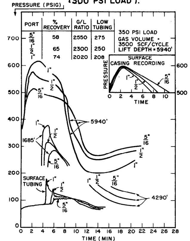
FIG. 17. COMPARATIVE PRESSURE RECORDINGS OF 1", 1/2" AND 5/16" PORTS.
