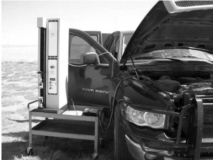
Portable tensometer under field power with laptop data download.
