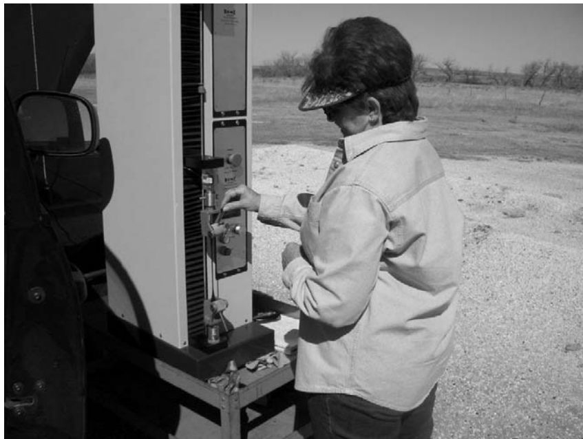
Samples tensile tested within minutes of removal from well.
