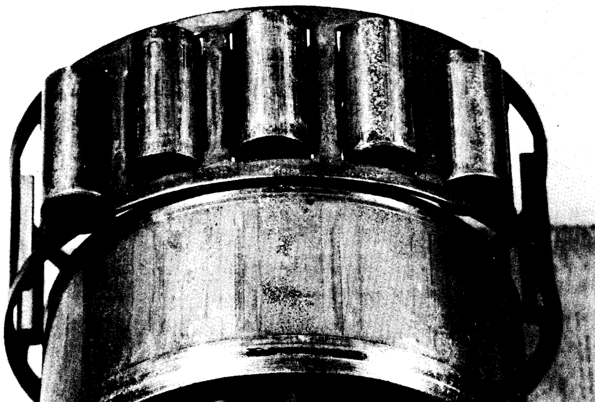
Fig. 6 Bearing failure, corrosion and wear, due to moisture in housing.
