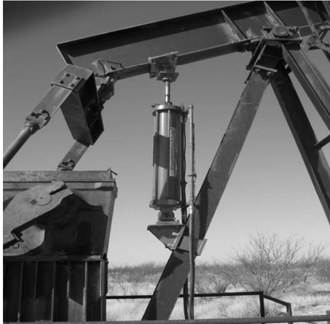
Figure 1 - Beam Gas Compressor Installation
