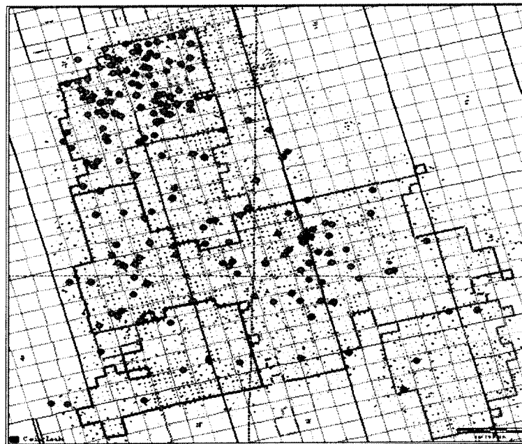
Figure 10 - Casing Failure Map with Outlined Pilot Area
