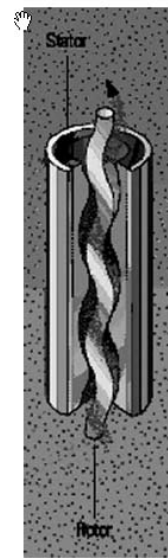
Figure 2 - PCP Pump Rotor and Stator
