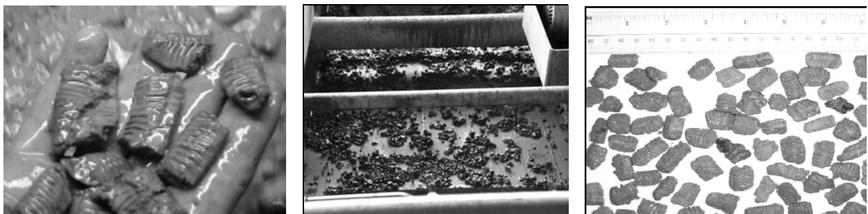
Figure 14 – Cuttings condition typified by use of NWBF (coupled with PDC bits) through reactive shales.
