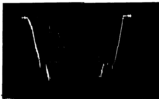
FIGURE 2—DRILLSTEM TEST PRESSURE RESPONSE, RADIAL FLOW ON INITIAL AND LINEAR FLOW ON FINAL BUILDUP
