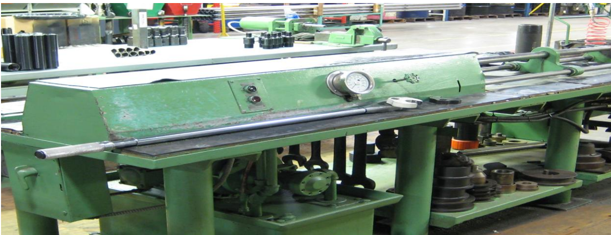
Figure 4 - Test machine used to measure required forces to pull downhole pumps from various seating assemblies.
