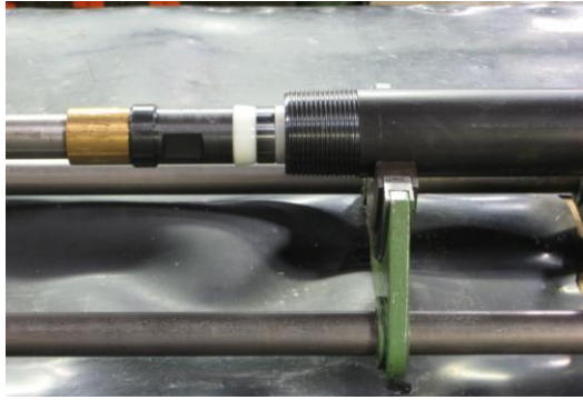
Figure 5 - Example test where the first ring or cup is being pulled from the seating nipple assembly.
