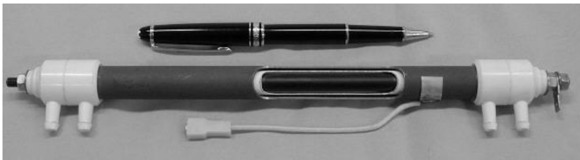
Figure 1 - ECA FEM-3 Technology (Flow-Through Electrolytic Module)
