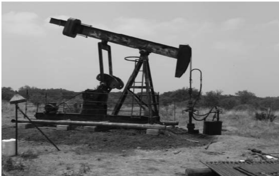
Figure 4 - CT-Lift System on Modern, Hydraulic Long Stroke Pumping Unit
