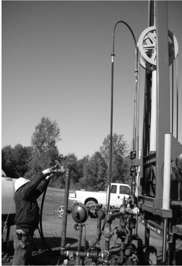
Figure 4 - CT-Lift System on Modern, Hydraulic Long Stroke Pumping Unit
