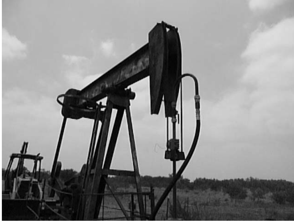
Figure 6 - CT-Lift System on Old Field, Old Pumping Unit
