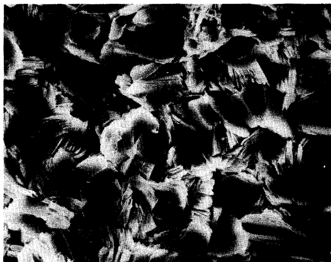
FIGURE 4—VIEW SHOWING DETAILED CRYSTAL STRUCTURE OF DIAGENETIC KAOLINITE EXTENSIVELY FILLING INTERGRANULAR AREAS. NOTE STACKED ("BOOK-LIKE") CRYSTAL PLATELET MORPHOLOGY AND MICROPORE SPACES BETWEEN CLAY CRYSTALS. SAMPLE DEPTH @ 12,943'; 1000X.
