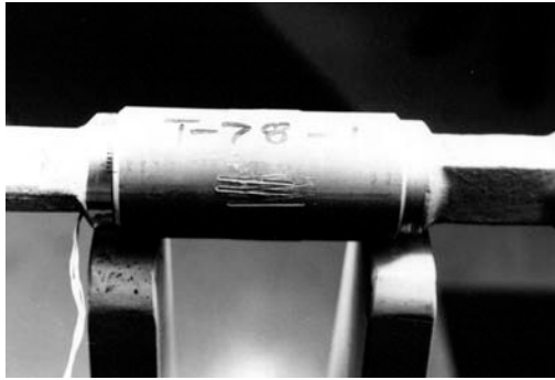
Figure 3 - Connection showing gauge leads. Figure 4 - Pre-stress results for C & K reruns for various diameters.
