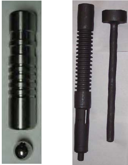
Figure 1 – Solid Ring Continuous Flow Plungers Pacemaker (Left) and RapidFlo (Right)
